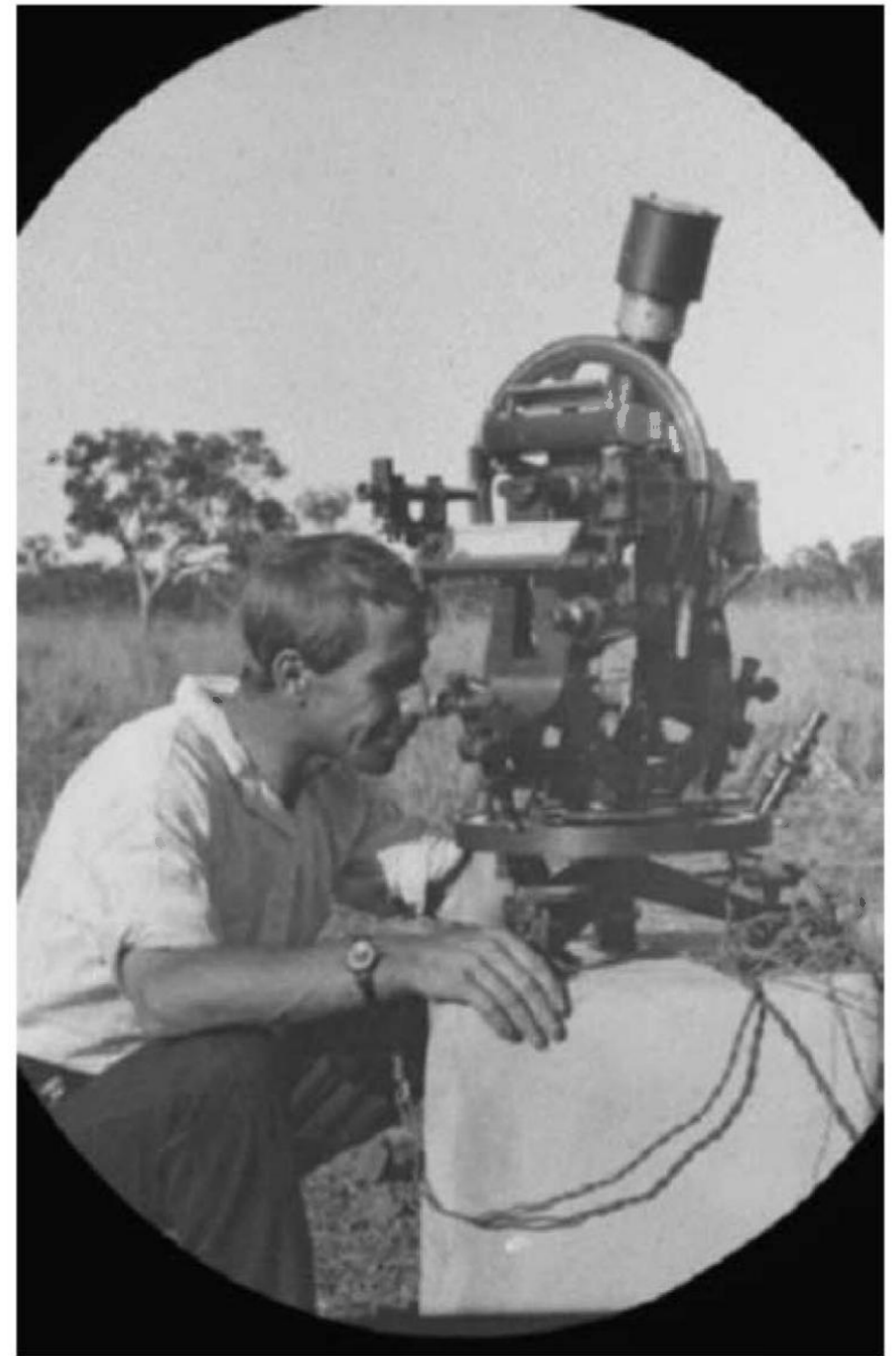
Figure 6. WA Government Astronomer Harold Curlewis using a 12 inch Troughton and Simms Theodolite #99 on the border determination expedition at the Austral pillars, c. 1921–22 (Landgate Files 8550/02 and 1191/97)
